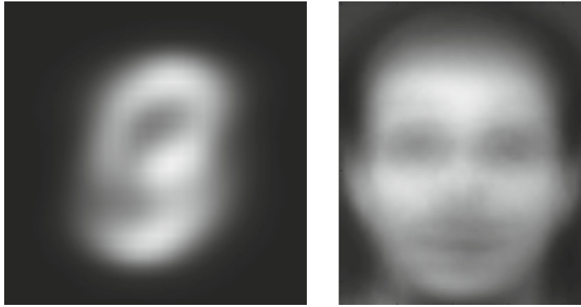
Fig. 9. “Mean faces”. On the left side there is a mean value of MNIST dataset, and the right image is FERET mean value.
